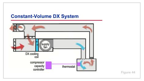
Again, a constant-volume system supplies the same quantity of air to the space and varies the temperature of this air to respond to changing loads.
